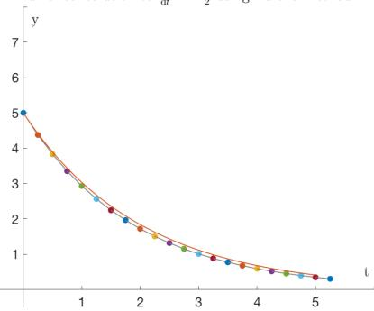
Unfortunately, small h means more iterations. Even more unfortunately, Euler's method is often not stable, meaning that the error in the approximation can quickly accumulate to such a size that the numerical solution diverges wildly from the true solution.
