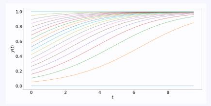
The differential equation is a rather famous one, and is used for population modelling. The y here represents the proportion of a population area that is filled. And the 0.5 in the RHS of the ODE is a parameter which determines the rate of growth/decline (e.g. try changing it to -0.5 to see decline).
